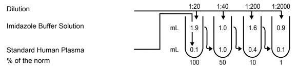
Additional dilutions can be prepared if necessary. Plot the measured coagulation times (ordinate) on log graph paper against the corresponding percentage factor activities (abscissa). The coagulation times are dependent on the measurement principle and thus also on the coagulation analyzer used. Therefore, each laboratory must establish its own reference curve.
