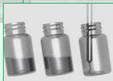
Tilted reagent vial positions to reduce reagent wastage
