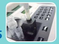
Dispense start reagent, measurement is started automatically. Result is displayed on the LCD screen or printed out automatically to an external printer
