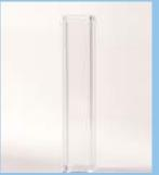
90 cuvettes - semi-permanent glass type, incubate in a dry bath for test reaction to take place.
